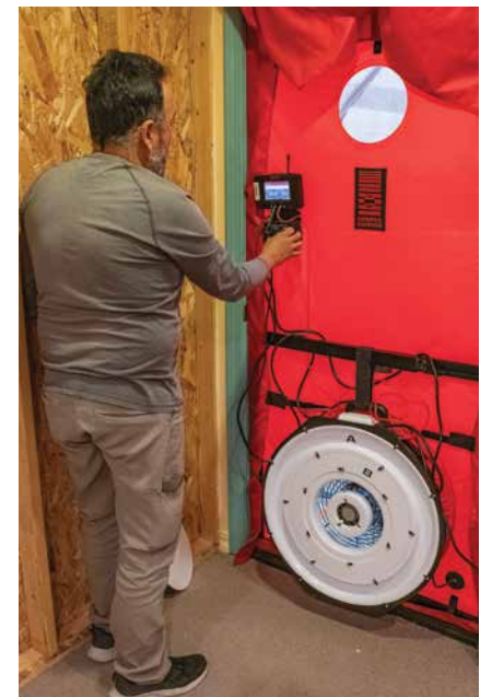
Left: Instructor Gerardo López and a student perform combustion analysis on a water heater; Above: López sets up a blower door in the ESA lab and performs a blower door test
