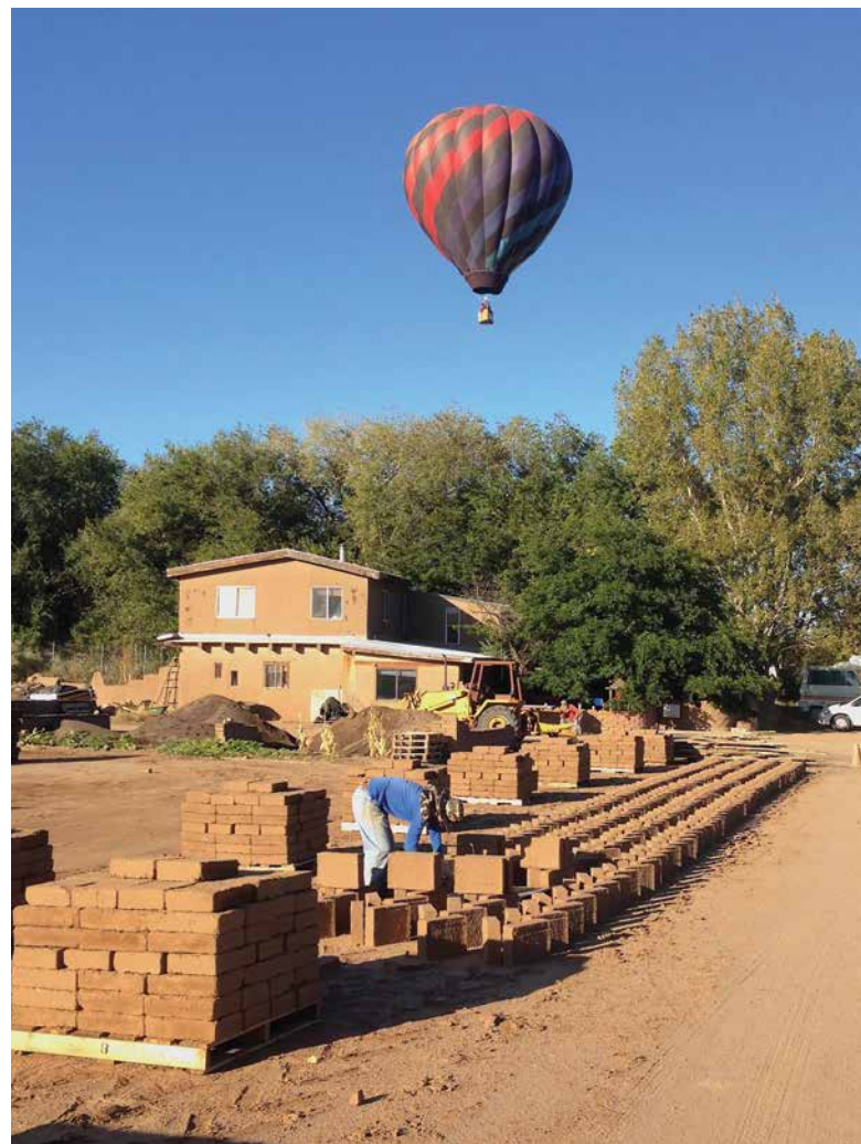
Adobe block making during the early morning hours. This is a view of the last production step of placing the dried adobes onto pallets before shipping to an eagerly awaiting construction site. This is New Mexico Earth Adobes, production yard in Albuquerque, one of the oldest adobe yards in the state.
