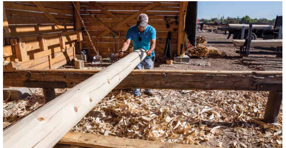
Peeling a viga at Wholesale Timber & Viga in Bernalillo, NM. WT&V recently joined the GoodWood program. Photo © Esme Cadiente
