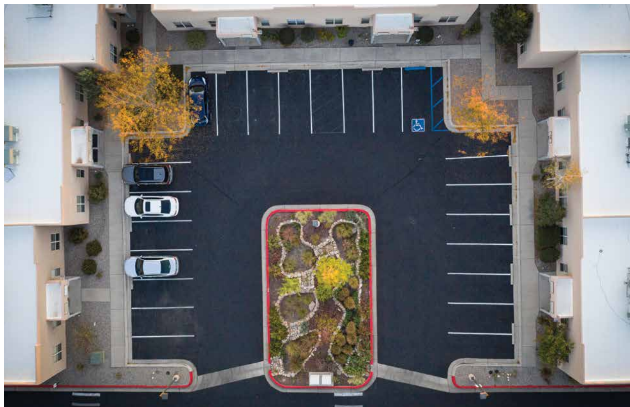
Top: A concept of a city as an ecosystem. Above: A raingarden built by The RainCatcher, Inc. in the middle of a business complex diverts stormwater through a series of basins, where it is purified by plants and fungi. The garden includes perennial edibles, including currents and oyster mushrooms.
